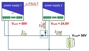
**Figure2** – System of 2 redundant power supplies: one of them was in failure in the Vout control, and Vout rises
