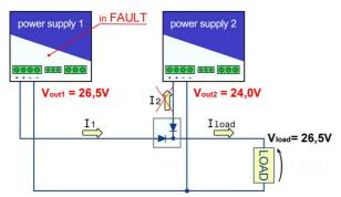
**Figure3** – System of 2 power supplies in redundancy: one has a fault in the control of Vout that cause che increase of Vout, but the power supply is equipped with overvoltage protection on the output.
