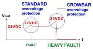
**Figure4** – Example of a standard overvoltage protection intervention, and CROWBAR intervention in an Advel SPS series power supply, output rated 24VDC
